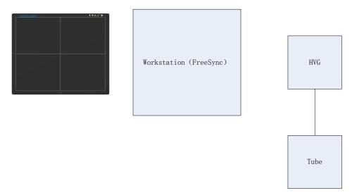
Workstation is a host PC device installed with iDetector and SDK. Chapter 3 has described how to establish connection between panel and Workstation. In FreeSync mode, User doesn't interact with Workstation. After shooting, images would be shown on screen immediately.
