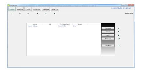
iRay provides test tools, such as iDetector for testing the basic performance of detector. It can connect the detector, acquire image, image correct and calibrate.
