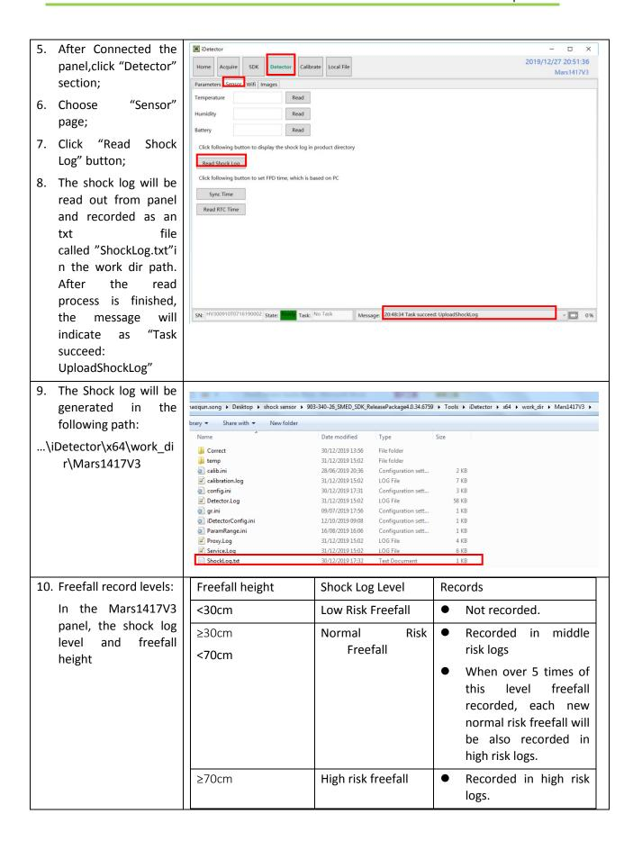
11. Open the Shock Log file, the log is indicated as shown in figure right.
