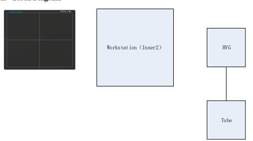
Workstation is a host PC device installed with iDetector and SDK. Chapter 3 has described how to establish connection between panels and workstation. In inner2 mode, workstation does not control x ray generator. Users would decide when to shoot x ray.
