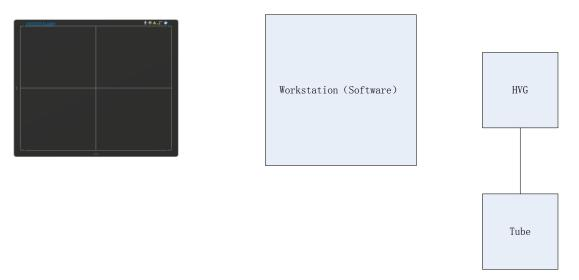
Workstation is a host device installed with iDetector and SDK. Chapter 3 has described how to establish connection between panels and workstation. In software mode, workstation does not control x ray generator. Users would decide when to shoot x ray.
